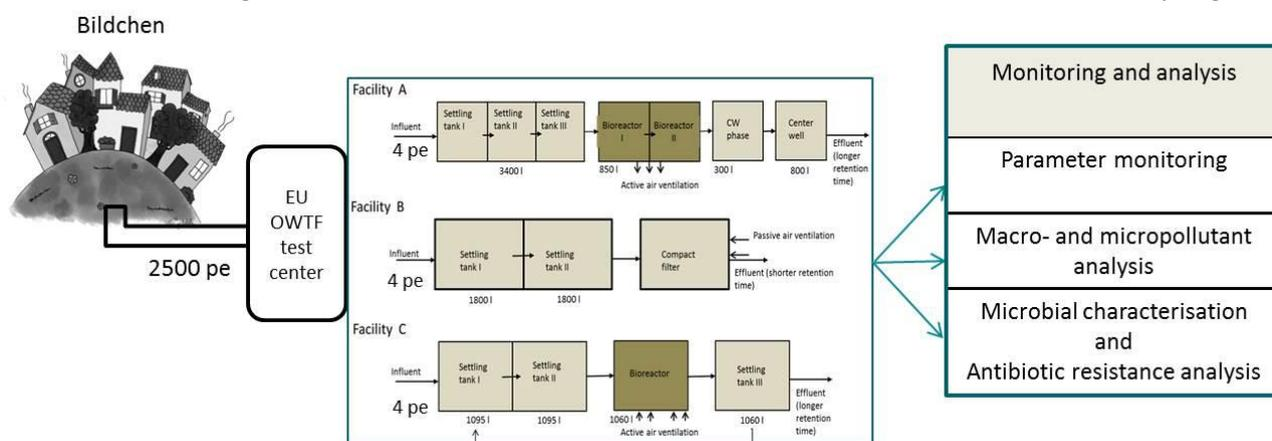
**Figure 1. Illustration of the test setup of onsite wastewater treatment facilities (OWTF) within BONUS OPTITREAT.**
